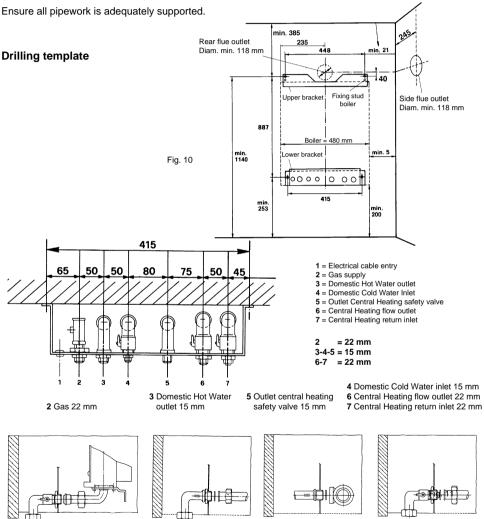
Important Note - Always use two spanners to prevent twisting of soft copper pipework.
