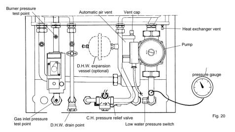
Remove the top front panel by gripping both sides and lifting forward away from main boiler assembly. Loosen the cap of the automatic air vent (fig. 20) and leave it loose.
