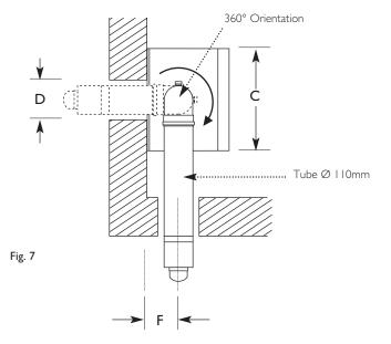
The 1.5° fall provided by the elbow is to allow condensate to run back to the boiler, for disposal through the condensate discharge pipe.
