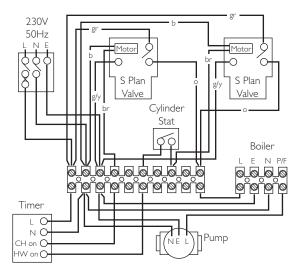
S Plan, Fully TRV'd System, CH Interlocked By Boiler Flow Switch Room Thermostat should not be fitted
