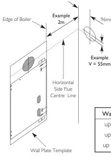
EXAMPLE: Boiler is 2 metres away from corner of wall, flue duct hole is 55mm up from horizontal side flue centre line. This will maintain the approx 1.5° backfall to the boiler.
