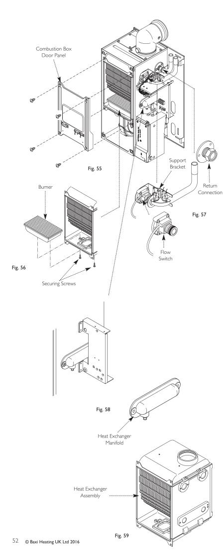
The burner and heat exchanger can be changed after removal of the combustion box door. To change the heat exchanger, the fan and burner must be removed first (see section 15.7 and 15.11).
