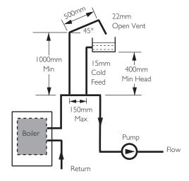
Fig. 10 Typical Low Head Installation
