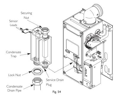
The removal of the fan is necessary to enable the changing of the injector pipe, condensate trap and gas valve (see section 15.7).
